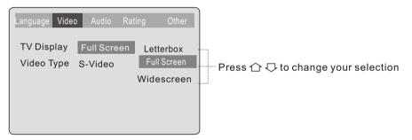
A. Press **ENTER** to confirm B. Press **OSD/SETUP** to exit the Setup Menu [Letterbox]----The full width of the picture is displayed on a standard 4:3 television, but black bars appear above and below the picture.
